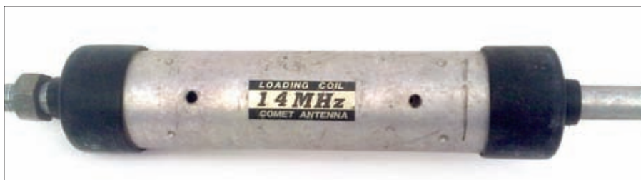
Enclosed traps, for tubular elements should be mounted with their drain holes at the lowest point.
