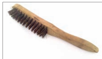
The steel-wire brush is a little 'savage' to use on aluminium elements, a brass-wire one is preferable.
